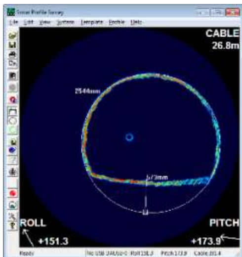
Profile of 100 inch diameter tunnel
